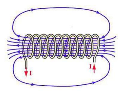
For a long solenoid (compared to its diameter), the magnetic field inside the solenoid is approximately uniform and approximately parallel to the axis, except near the ends of the solenoid. Outside the solenoid, the magnetic field looks like the field of a physical dipole, with the North pole at one end of the solenoid and the South pole at the other end.
