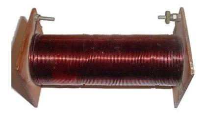
Each wire loop in this coil acts as if it was a separate circular wire carrying the same current I — the current in the coiled wire — and the dense enough array of such loops may be approximated by a *cylindrical current sheet* with the current density
