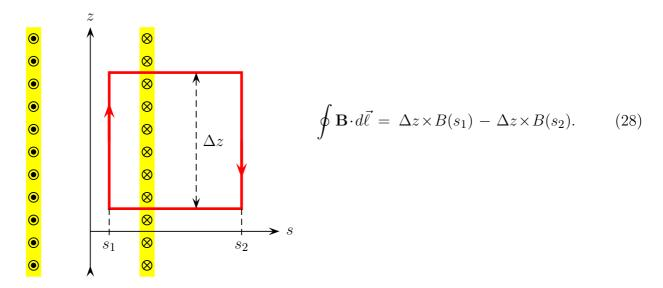
The net current through this loop includes all the solenoid's coils crossing the loop (28), thus
